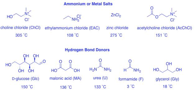
**Figure 1.** Example DES components and their pure-component melting points. At the eutectic ratio, the salts and hydrogen bond donors form liquids at room temperature or slightly above room temperature
