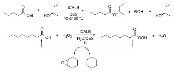
**Figure 2.** Examples of reactions in DES's. The top reaction is a transesterification reaction with no water present; the bottom reaction is a perhydrolysis in a combination of DES and water.
