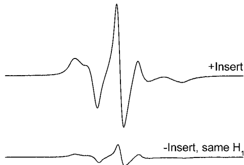
FIG. 7. EPR spectra acquired for a lipid sample: fatty acid spin label 5-SASL in DOPC lipids. The quantity of 5-SASL in the sample is approx. 0.4 nmoles. In the TE cavity with the insert, P = 0.63 mW, H_1 = 123 mG (top). In the TE cavity without the insert, P = 15.94 mW, H_1 = 121 mG (bottom). Sample length, 2.2 mm; volume, 0.3 \mu\text{L} . Experimental conditions: gain 80 dB ( 2e5 ), time constant 41 ms, sweep 110 G/42 s, 30 scans acquired for each trace.
